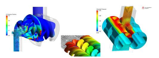
SCORG<sup>TM</sup> will minimise efforts and maximise efficiency of the analysis and design of screw machines and other rotary positive displacement machines.
