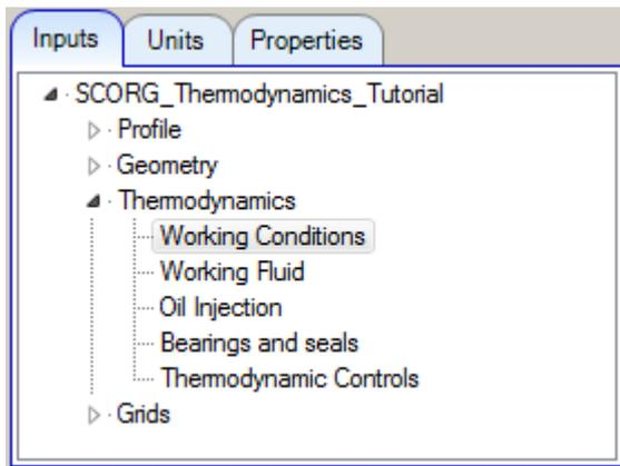
The setup for Thermodynamic calculation is performed through the Input controls shown in the control window on the left.
