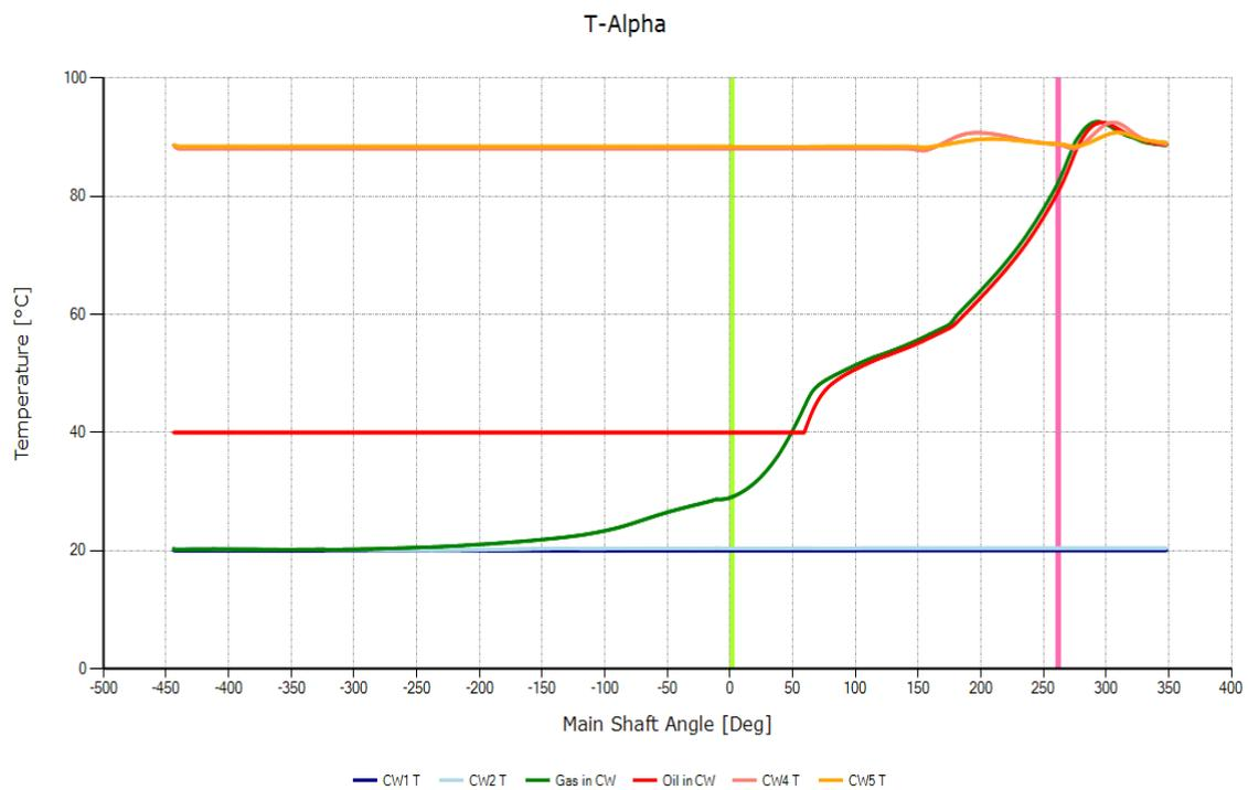
Notice the red line which represents the oil in the working chamber. Oil is injected at 60 deg and is used to cool the air. Despite the discharge pressure reaching almost 9 bar, the discharge temperature is around 80 deg C.
