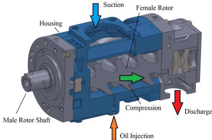
Figure 1.1 Oil injected twin screw compressor cross section
