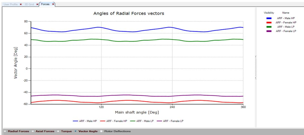
Please note that the forces on bearings depend on the relative position of bearings to the machine low and high pressure ends. The position of bearings is set using the Geometry->Restrains table below:
