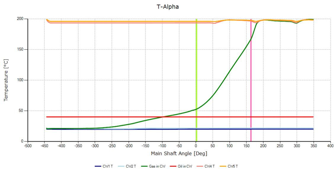
The above two diagrams show Pressure change with the angle of rotation and the temperature change with the angle of rotation respectively. The green line marked with CW represents the main working chamber.
