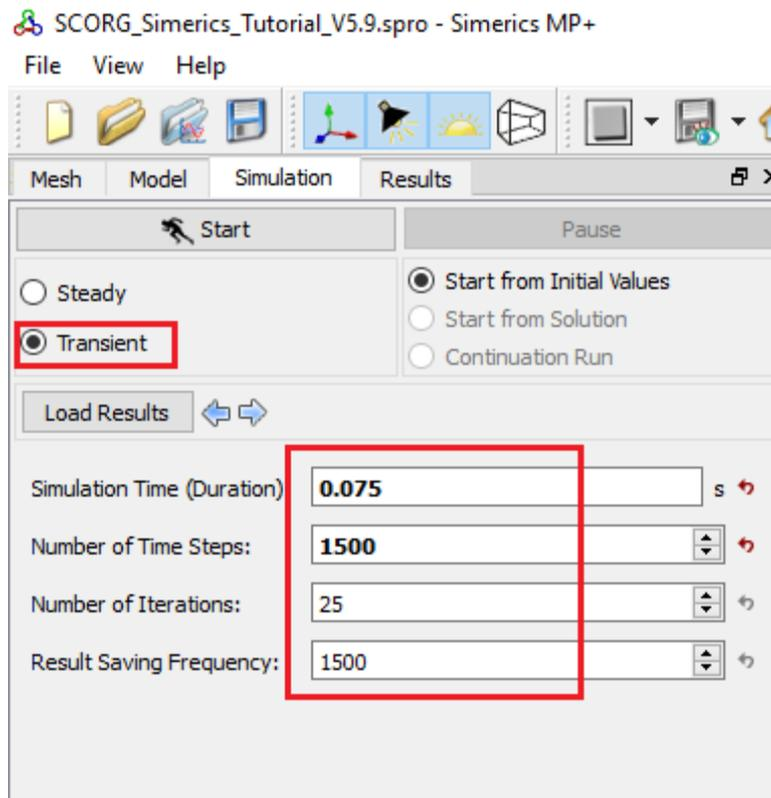
The time step size is controlled by the number of divisions used for angular discretization during grid generation in SCORG.
